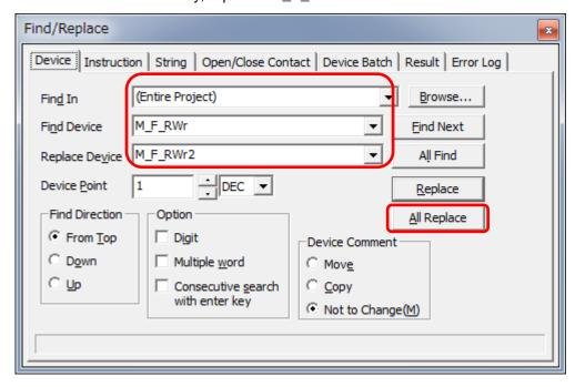
By performing the steps above, the CC-Link IE field master/local FB can be used for the second module.
