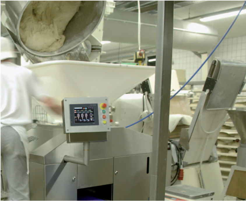
Variable speed drives and servo control technologies provide accurate scaling of the dough
