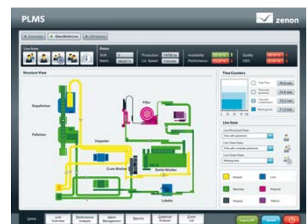
A production line management system with zenon
