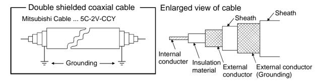
The 5C-2V connector plug is applicable to double-shielded coaxial cable. Connect the 5C-2V connector plug to the coaxial cable inside a double-shielded coaxial cable. Ground the shielded part outside a double-shielded coaxial cable as shown in the above figure.
