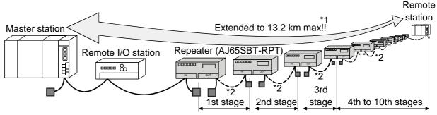
\*1 Max. transmission distance at a transmission speed of 156 kbps.
