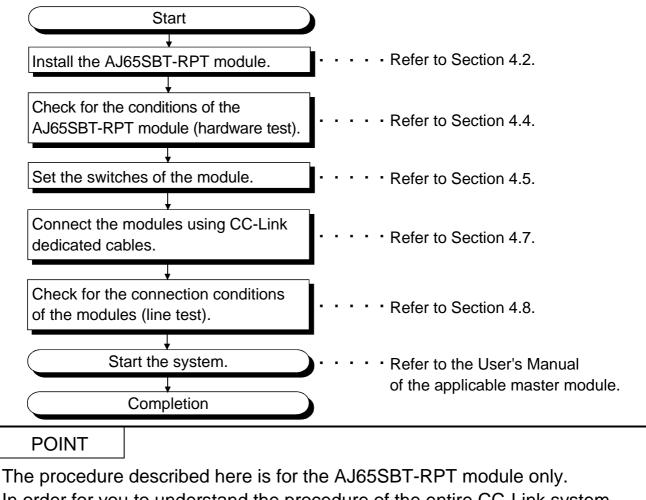
In order for you to understand the procedure of the entire CC-Link system, refer to the User's Manual of the applicable master module.
