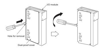
Insert the tip of a flathead screwdriver into the hole, and gently tilt the screwdriver to pry the cover off. (See the figure above.)
