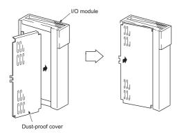
Insert one side of the dustproof cover into the groove of the module (on the connector or terminal side) first, and push the other side of the cover in the module until it locks into place. (See the figure above.)
