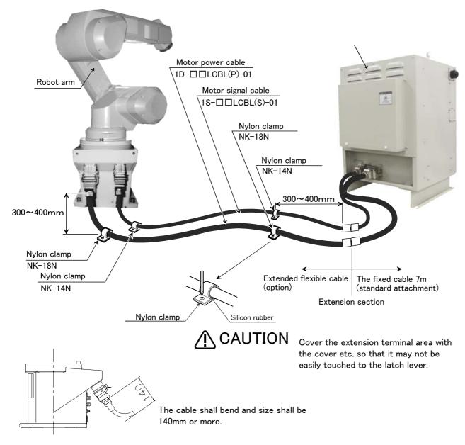
Fig.2-9: Fixing the flexible cable
