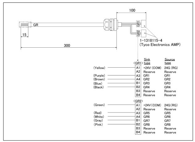
Fig.2-11: Outline dimensional drawing and pin assignment
