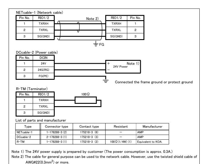
Fig.3-23: Spacifications for the connection cable
