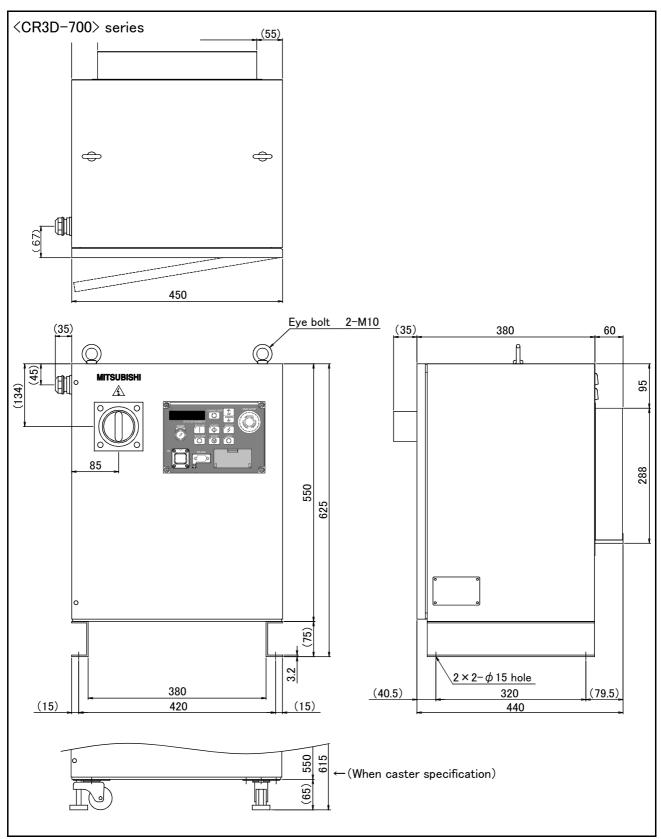
Fig.3-5 : Outside dimensions of controller(CR3D-700)
