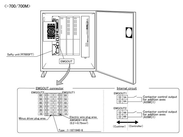
Fig.3-16: EMGOUT connector (CR3D-700/700M)
