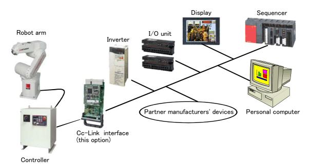
Fig.3-29: Example of CC-Link Product Configuration
