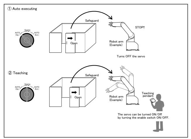
Fig.3-13: Door switch function
