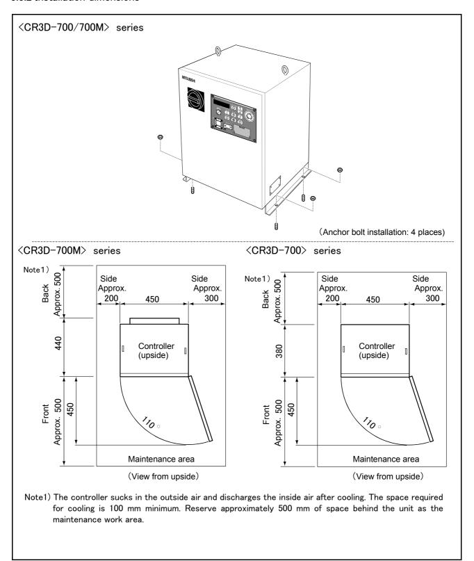
$Fig. 3-8: In stallation of controller \ (CR3D-700/700M)$
