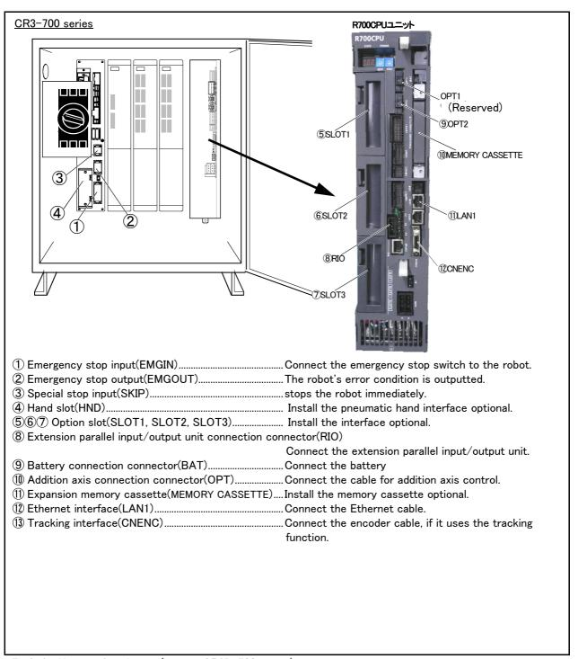
Fig.3-4: Names of each part (interior CR3D-700 series)
