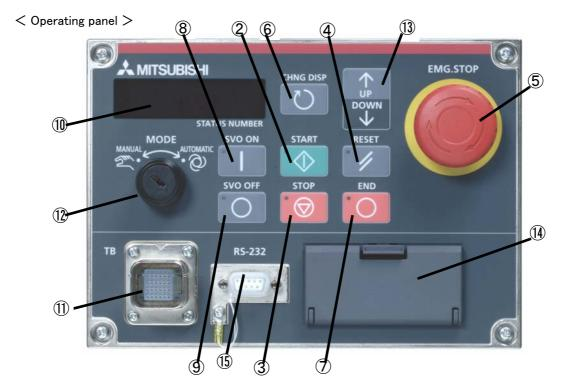
Fig.3-1: Names of controller parts
