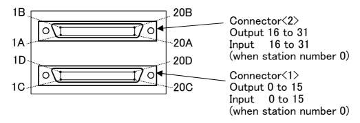
Fig.3-21: Pin layout of connector
