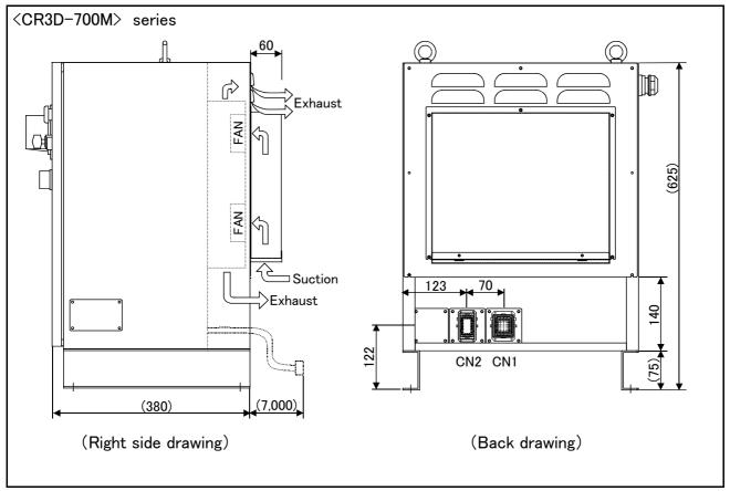
Fig.3-6: Outside dimensions of controller (CR3D-700M Supplement)
