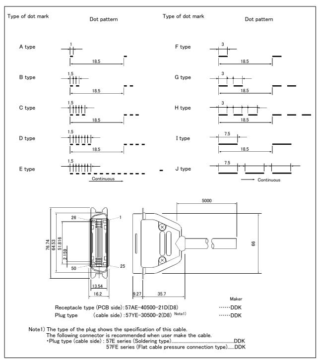
Fig.3-27: Connections and outside dimensions
