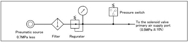
Fig.2-8: Air supply circuit example for the hand
