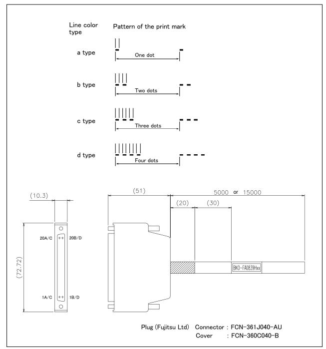
Fig.3-22: Connections and outside dimensions
