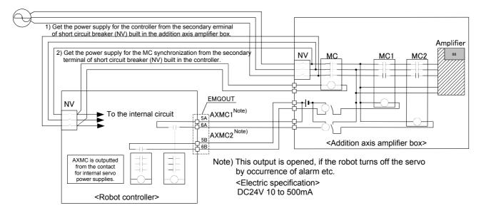
Fig.3-15: Example of circuit for addition axes of Magnet contactor control output
