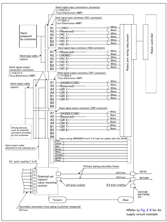
Fig.2-7: Wiring and piping system diagram for hand and example the solenoid valve installation(Source type)
