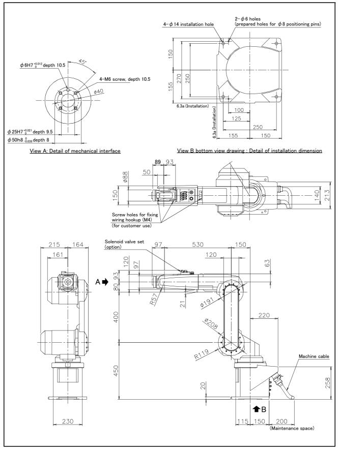
Fig.2-3: Outside dimensions: RV-18SD-S/18SDC-S
