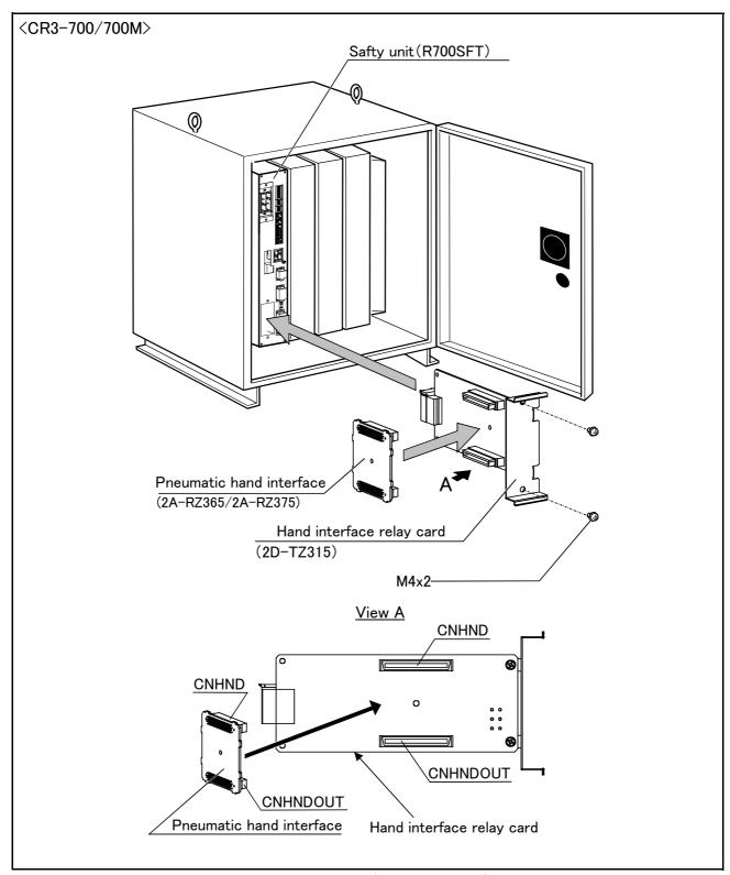
Fig.3-19: Installation of the pneumatic hand interface (CR3D-700/700M)
