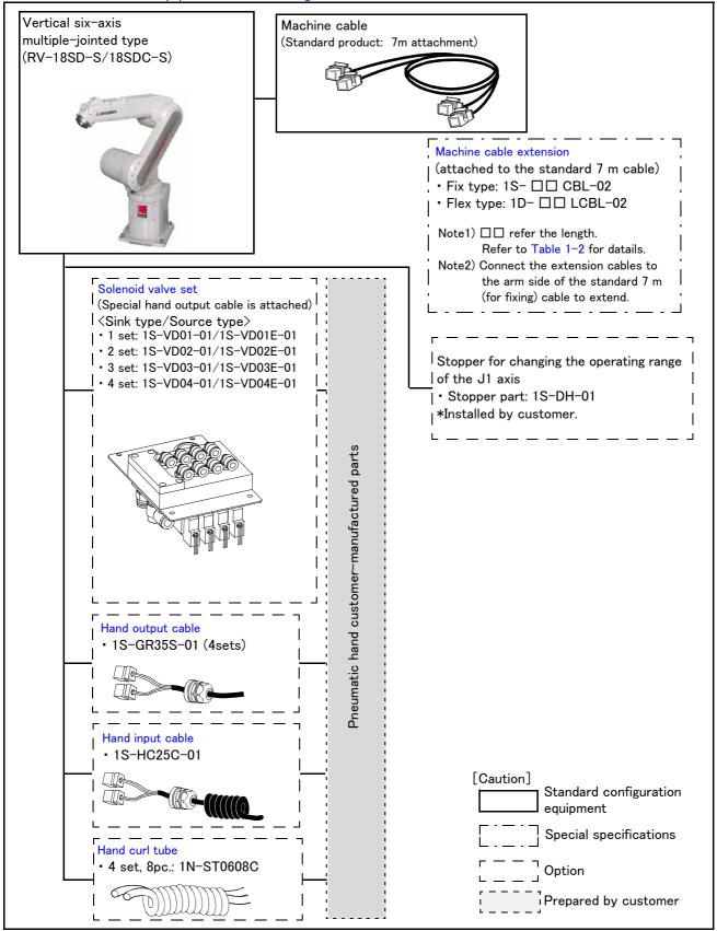
Fig.1-1: Structural equipment (Robot arm)
