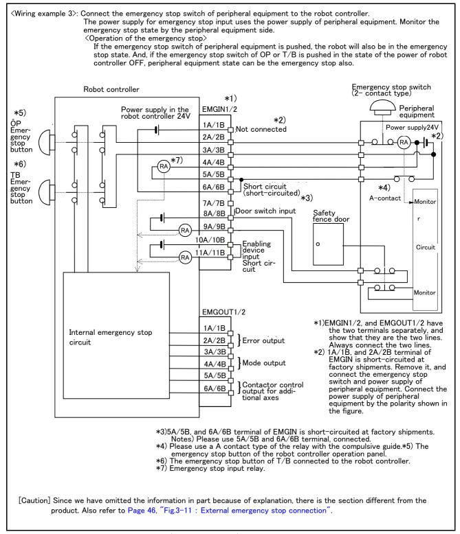
Fig.6-3: Example of safety measures (Wiring example 3)
