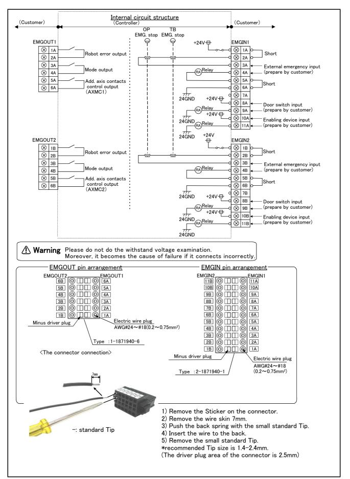
Fig.3-11: External emergency stop connection
