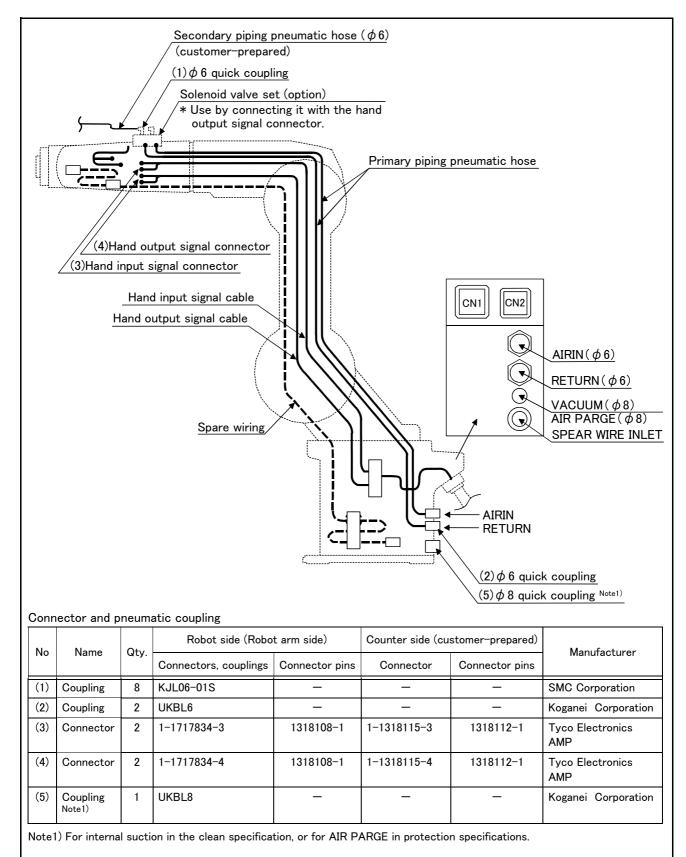
Fig.2-5: Wiring and piping for hand
