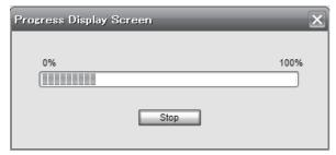
Completing the one-touch tuning starts writing tuning parameters to the servo amplifier. "0 0 0 0" is displayed at status in error code. In addition, settling time and overshoot amount will be displayed in "Adjustment result" after adjustment.
