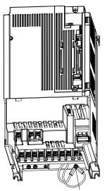
Built-in regenerative resistor lead terminal fixing screw
