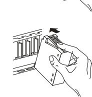
② Push the module in the direction of the arrow to load it into the base unit.
