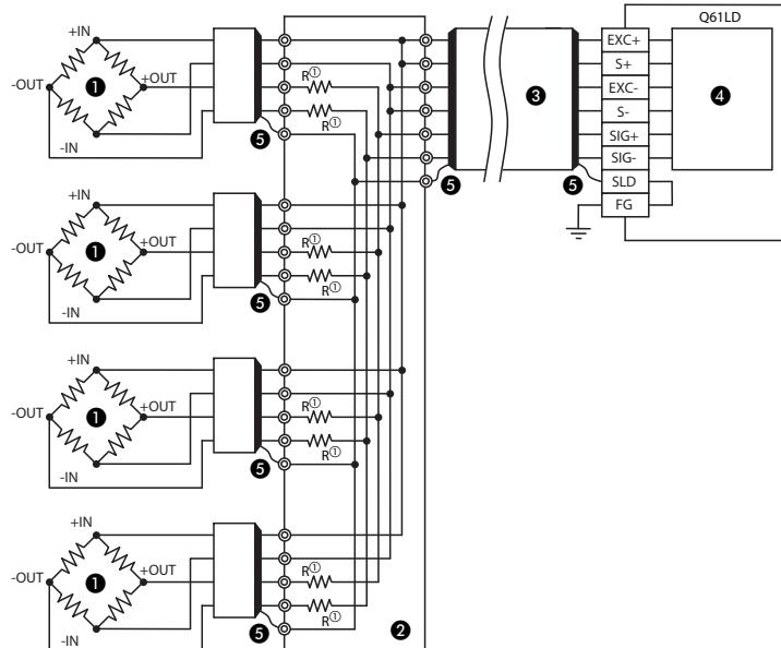
① The average resistance ( $R$ ) in the parallel circuit requires  $300\Omega$  to  $500\Omega$  relative to the electric power. The resistors require a low temperature coefficient of resistance. When the output voltage is adjusted for load cells connected in parallel, the resistance ( $R$ ) is not required. /
