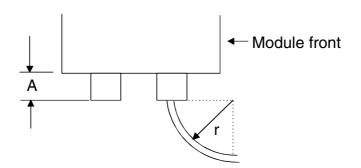
3) The optical fiber cable is wired in the following manner.
