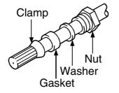
c) Cut the external conductor, insulation material and internal conductor to the dimensions shown below. However, cut the external conductor to the same dimension as the tapered section of the clamp and smooth it down to the clamp.
