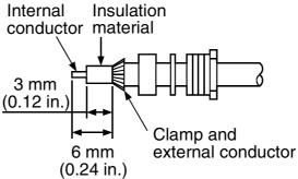
d) Solder the contact to the internal conductor.
